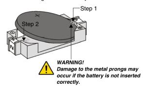
Battery type: One 3V lithium battery (CR2032)
